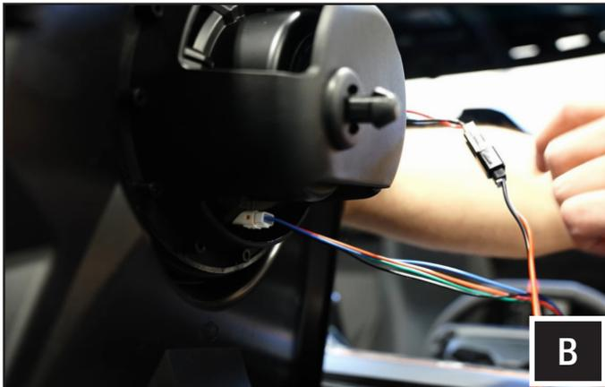
B. Plug in speaker connector of B-H1385 to the driver and passenger side dash panel speakers.
