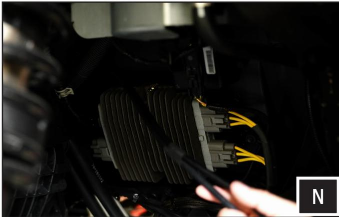
N. Split the B-H2936 rear speaker harness to the passenger and driver side along the rear firewall. Zip tie the cables to the factory harness and avoid hot or moving parts.
