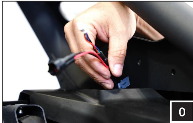
O. Run the driver and passenger side speaker harness through the plastic panel by the B-pillar.
