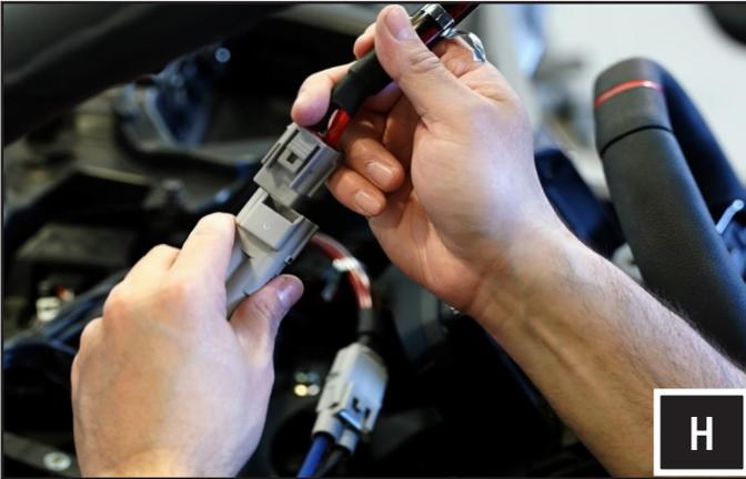
H. Plug in the power connector of the amp to the power cable.
