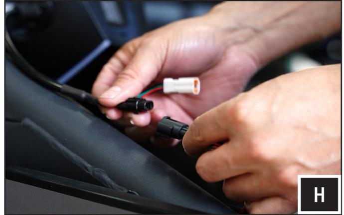
I. Plug in the speaker pod audio connector to the B-H2936 rear speaker Y harnesses.
