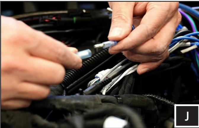
J. Plug in the amplifier turn-on bullet connector to the turn-on delay module output wire. See page 4 for reference.
