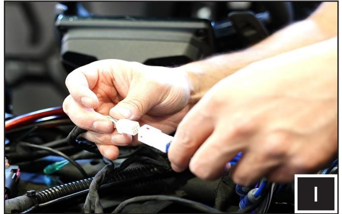
I. Plug in the factory radio output connector to the 8-pin speaker input connector of the amplifier.
