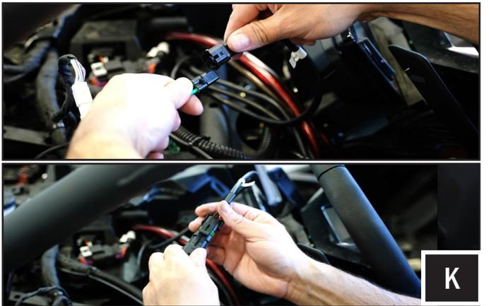
K. Plug in the amplifier's front speaker output to the B-H1385 "Y" harness and the rear speaker outputs to the B-H1913, 4-pin audio extension harness.
