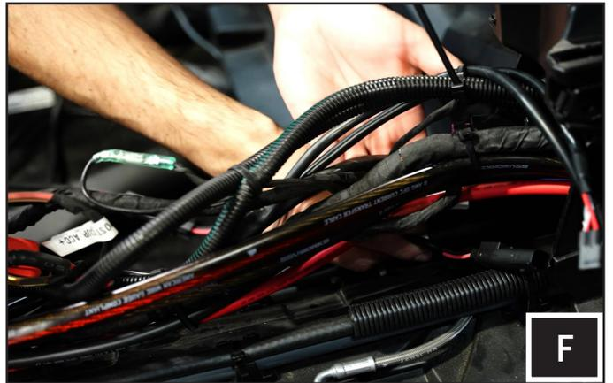
F. Run the rear speaker cables along the passenger side of the center console. Use zip ties to tidy up the install.
