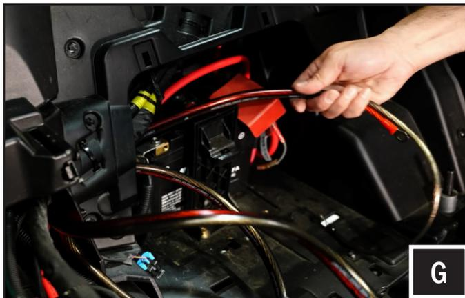
G. Route the power cables along the driver side center console from the battery location towards the driver side dash.
