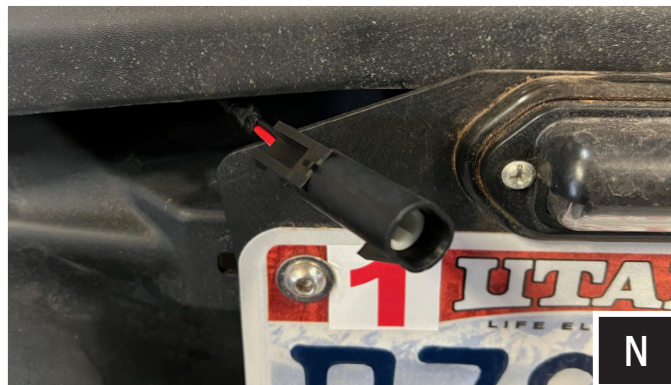
N. Route the license plate light power connector towards the license plate location. SSV license plate frame with LED light is sold separately. Contact SSV customer service at (818)991-1778 for more information.
