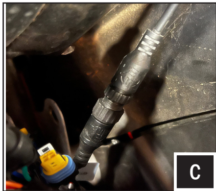
C. Plug in the controller cable, front turn signal extension cables (B-H2959) and rear turn signal harness (B-H3204) to the TANGO2 main harness (B-H2939).
