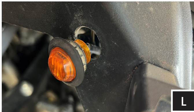
L. Insert the LED turn signal lamp into the hole and push in to lock in place. Repeat steps K and L for the other side.
