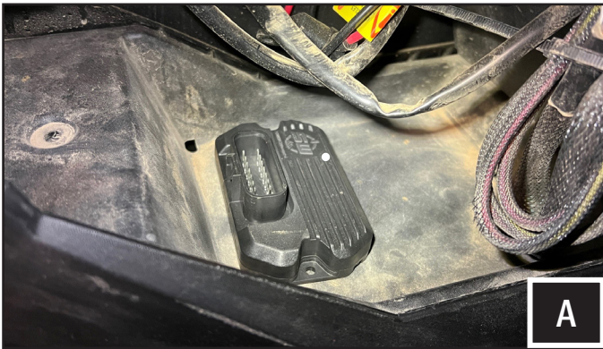
A. Find a suitable mounting spot for the Tango2 brain module preferably near a power source and within the cable length of the turn signal rocker switch. Screw the module to a flat surface or zip tie it to a wire loom. The module was mounted on the front section of the center console in this sample installation.
