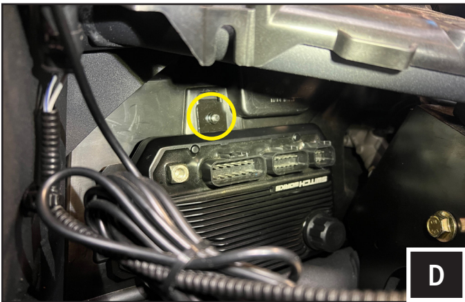
D. While holding the ALPHA12 brain and bracket with your right hand, use your left hand to screw in the (2) factory bolts removed in step B.
