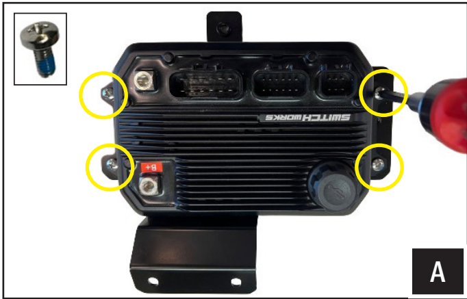
A. Mount the ALPHA12 Brain module to the Mav R brain module bracket using (4) M5x10mm Phillips screws [B-S1158].
