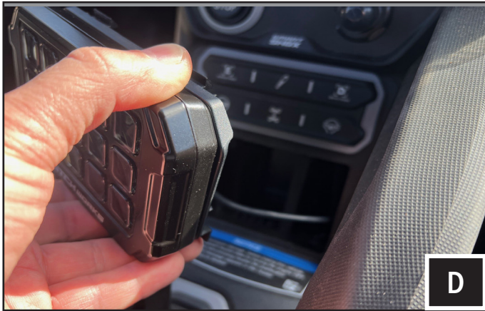
D. Run the cable towards the bottom of the dash. Line up the bottom side of the controller to the dash opening and push in the top to lock it in place.
