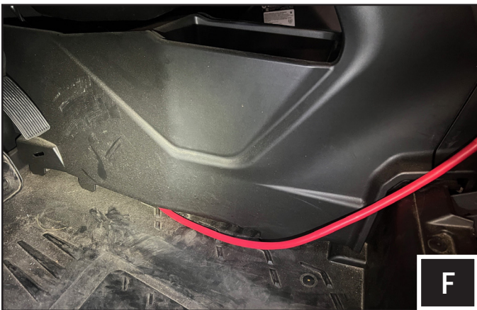
F. Run the power cable to the battery behind the driver seat.
