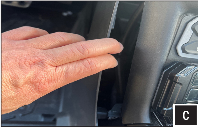
C. Remove the driver side center dash side panel. It is held by clips.
