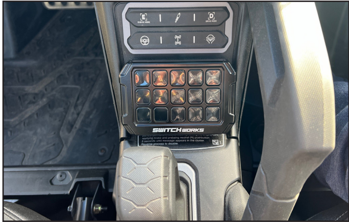
Completed installation of 15-Button Controller.
