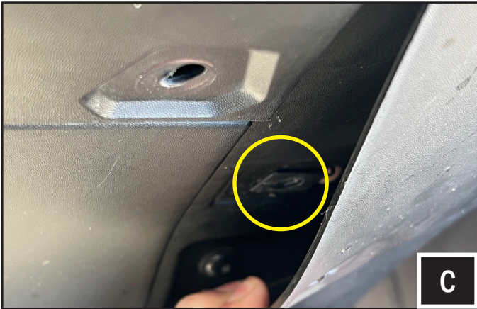
C. Remove the (2) factory U-Nuts that were used to fasten the (2) bolts removed in step B.
