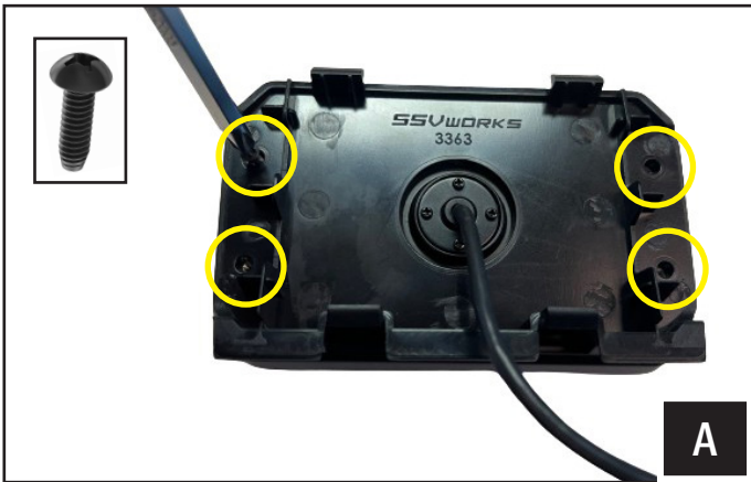
A. Mount the 15 button controller to the Mav R Push-In dash panel using the provided (4) 4-40x0.375 thread cutting screws [B-HP3356]
