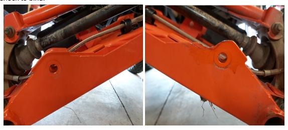
\*\*\* Shock mounts can be "smashed" from the factory requiring the mounts to need spread for proper shock fitment\*\*\*
