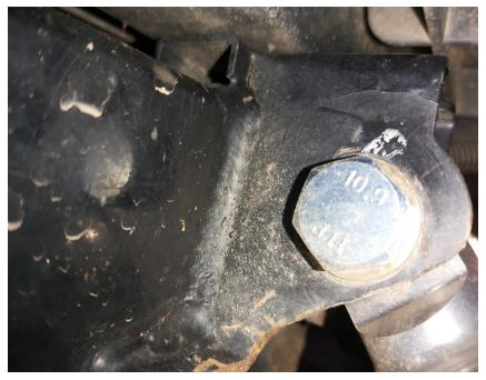
\*\*\* Shock mounts can be "smashed" from the factory requiring the mounts to need spread for proper shock fitment\*\*\*
