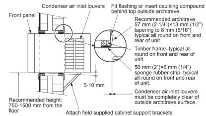
• When constructing a timber frame, arrange so that the outside rear of the air conditioner is between 5 and 10 mm lower than the front of the unit This allows condensed water to drain off outside the room If the inside of the air conditioner is lower, condensed water and rain may flow into the room.
