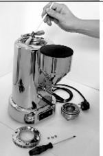
Make sure that everything is very clean when reassembling the parts. There should be no coffee grounds remaining on the threads. Otherwise you will not be able to put the parts back together again correctly.
