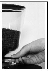
Loosen the screws of the grinder dial with an Allen wrench (2.5mm).
