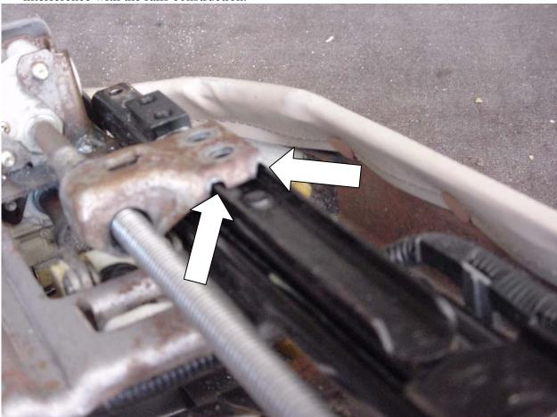
2. Using 2 8Mx10 bolts, bolt the bracket to the following nut assembly tight enough to hold its position but still allow for movement.
