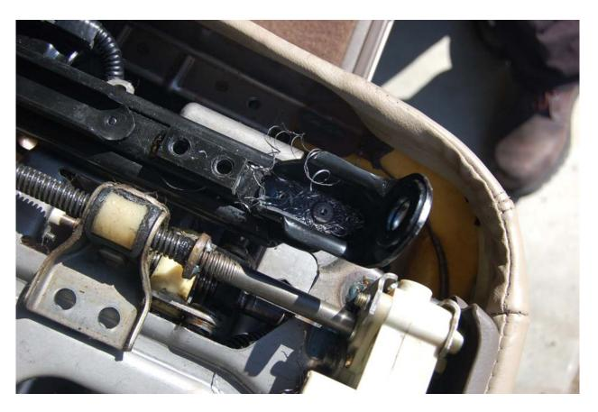
This shows the two 1/8" pilot holes that gets drilled into the rivet and spot weld.
