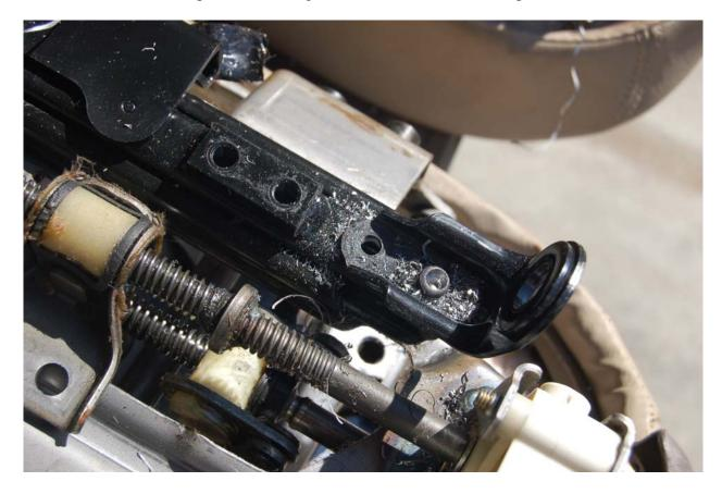
Here you can see that the pilot holes have been drilled out with a ¼" drill bit. On the rivet you only drill down to the surface of the foot and then knock off the head with a hammer to preserve the original hole.
