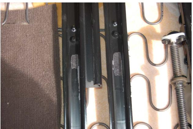
2. On the upper rail at the front there are 3 12mm bolts. The rear one needs to be removed and replaced with the 8MX16 flat head bolt. You will need to countersink the hole for this bolt as the rollers will now travel over the top of it. The next series of pictures shows the bolt that gets removed, countersinking the hole and the flat head screw in place flush with the rails surface. The last picture shows the counter sink bit used.
