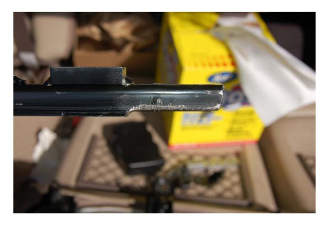
Remember, the rails get ground on the inside of their perspective sides. So if holding the rails side by side the ground edges should face each other.
