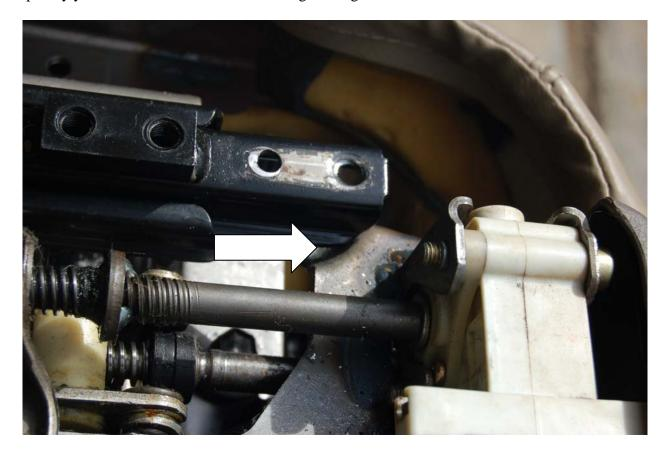
The next series of pictures shows a stock rail and then the material removed to allow it to not contact that area
