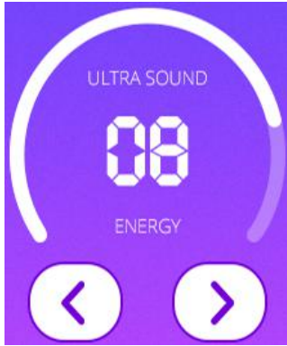
energy level and adjusting buttons
