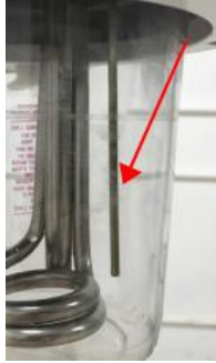
Water Level Detector
