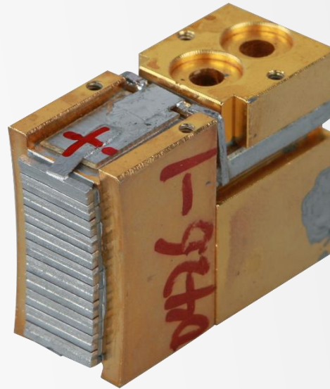
Other product Encapsulated with Indium, target bar is exposed
