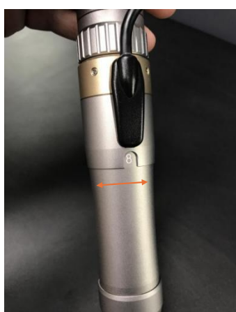
Twist left or right to select desired spot size
