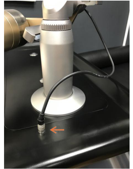
Step 10. Plug in cable from main arm into machine
