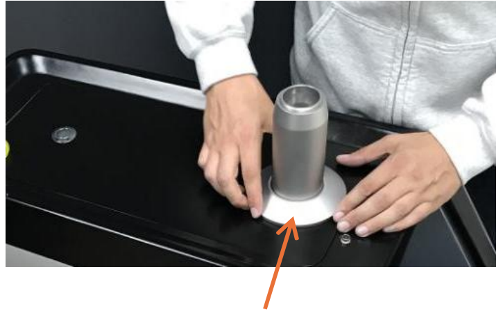
Step 2. Place locking plate (8) over the laser entrance and screw into place until tight
