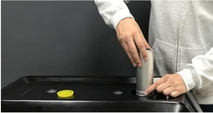
Step 1. Screw laser entrance (2) into the machine
