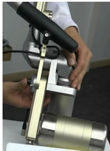
Step 12. Twist button (3) and push in to adjust bob-weight position to 90°
