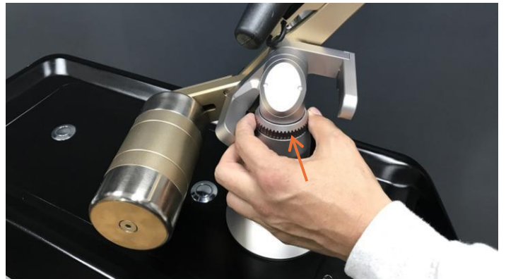
Step 4. Screw main arm locking plate (6) onto laser exit window
