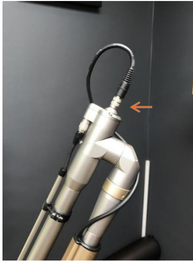
Step 9. Plug in cable at top of laser arm
