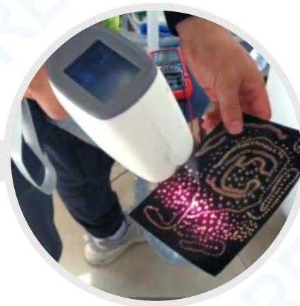
The third inspection: Light spot inspection (burning test)
