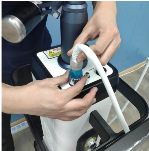
Step4: Align the galvo with the light guide arm.
