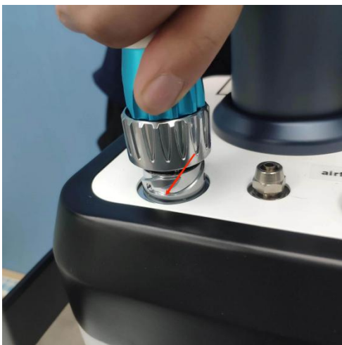
Step5: Install the galvanometer signal line.
