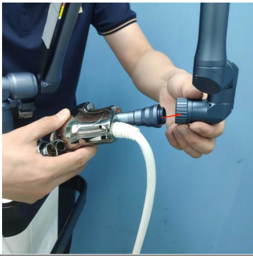
Step4: Align the galvo with the light guide arm.
