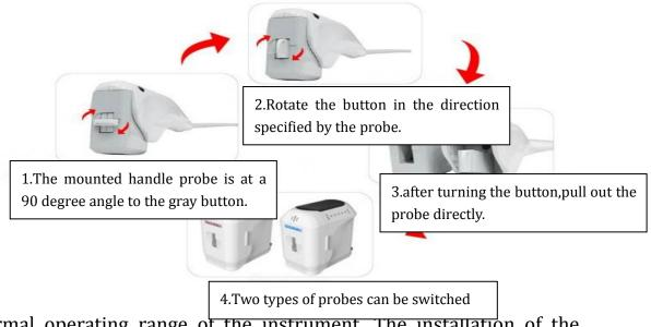
normal operating range of the instrument. The installation of the probe is shown below.
