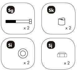
Attach 1 seat and back (K) to left and right arms (H & I) with 2 bolts (Sg), 2 plastic washers (Sk), 2 large metal washers (Si) and 2 nuts (Sj). Note: the side of the seat with "front" label should be in accordance with the side with label of the arm. Securely tighten all bolts for this step.
