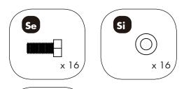
Attach 1 side panel (B) to the leg posts (A) with 8 bolts (Se), 8 large locker washers (Ss) and 8 large metal washers (Si). Do not tighten completely.
