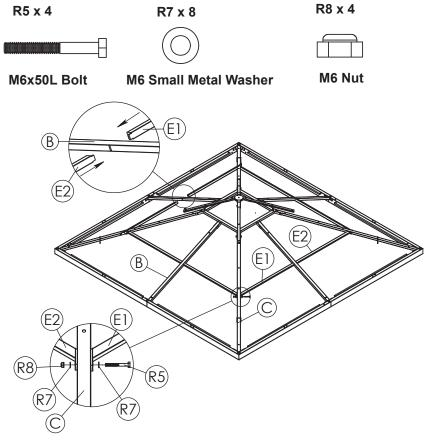
Insert to connecting bar (E1,E2) to the opening of the short canopy frame bar (B). Tighten all bolts of steps above.
