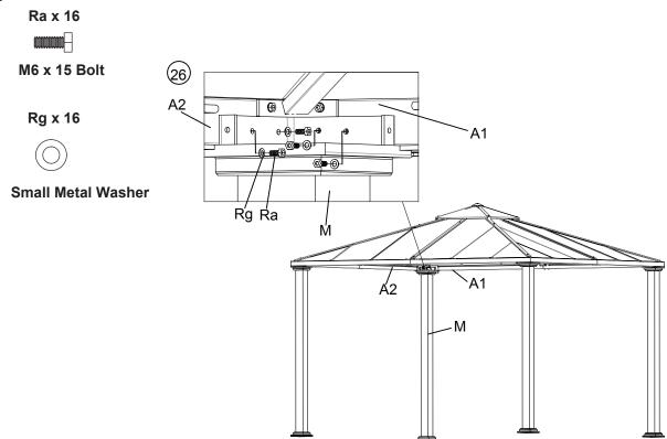
Repeat procedure for the remaining three leg posts.
