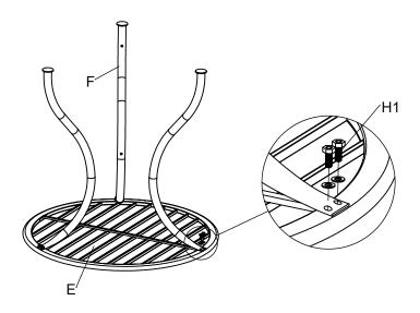
Do not tighten completely. Repeat procedure for the other two legs.
