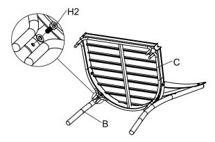
Do not tighten completely. Repeat procedure for the other side.
