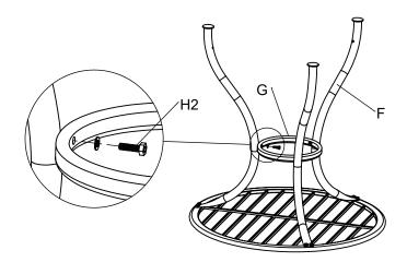
Do not tighten completely. Repeat procedure for the other two legs.
