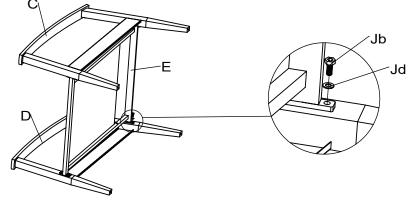
Don't tighten completely. Repeat procedure for the other side.
