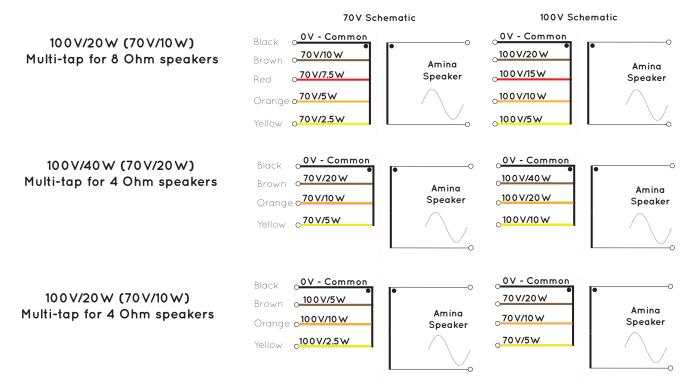
To limit the risk of spurious noise from loose cables, please carefully dress and tie back the unused input taps using a cable tie. See diagram below.
