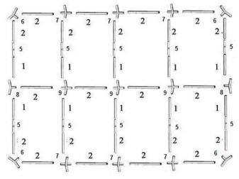
Model shown is 5x8m tent. Simply increase or reduce to the desired length by adding or reducing 2 metre bays using parts 1,2,5,7 and 9.
