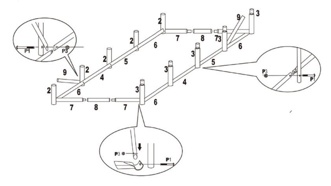
Loosely assemble complete frame, before tightening all bolts in final position. Fit all Horizontal and diagonal bars on the INSIDE of the tunnel Arch.
