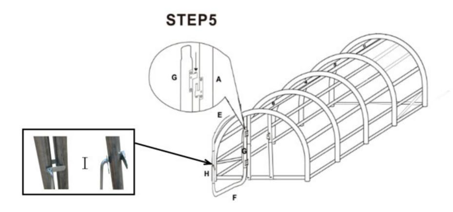
Fit all Horizontal and diagonal bars on the INSIDE of the tunnel Arch.
