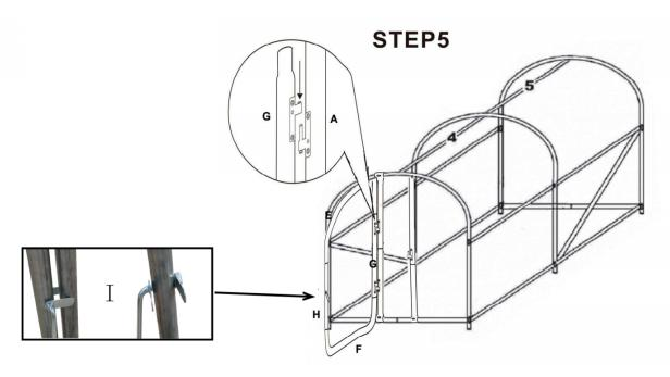
Next thread through the locking screw and tighten.
