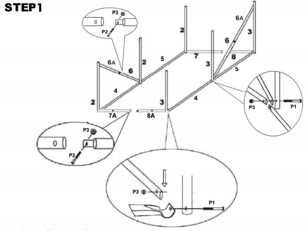
Loosely assemble complete frame, before tightening all bolts in final position.
