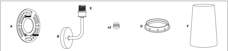
1. Measure area and determine desired mounting height. 2. Detach mounting plate [A] from backplate [B]. **3.** Mounting plate [A] will attach to junction box. 4. Install light to wall. Linea Lighting recommends installation by a qualified electrical professional. Backplate nuts [C] are used to tighten light to wall. 5. Remove socket ring [D] from socket [E]. 6. Slide fabric shade [F] onto socket [E] and tighten with socket ring [D]. Install bulb 60W max (not included).
