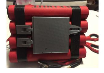
Using the hole on the back door as a reference, stick the ushaped metal on the black tape. Press firmly for a minute.
