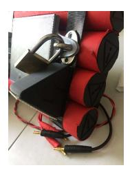
Take the triangle piece out. It is 3d printed and comes with a velcro tape. Remove the sticker on the velcro tape and place it just below the U shaped metal. Do not press firmly yet.
