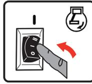
8. Push the battery power restore switch for about 3 seconds and then release.
