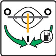
5. Flip the engine switch to the "RUN(I)" position.
