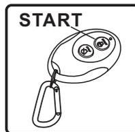
6. Push and hold the program button approximately 3 seconds until the indicator light turn off. The generator is now programmed to start remotely.
