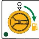
3. Turn the fuel selector switch to GAS position
