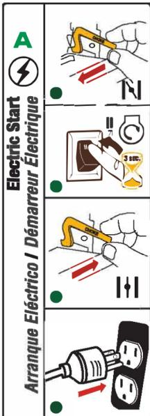
4. Move choke lever located on engine to START position
