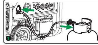
1. Connect the regulator to both LPG cylinder and generator.
