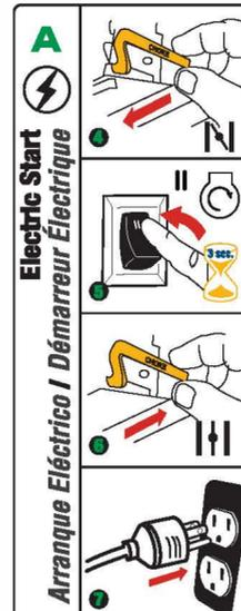
4. Move choke lever located on engine to START position
