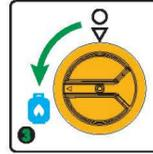
3. Turn the fuel selector switch to LPG position
