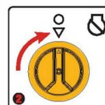
Turn the fuel selector switch to OFF (O) position
