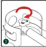
2. Make sure the LPG cylinder knob is fully closed
