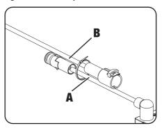
2. Insert the male connector of cable A into female connector of cable B.
