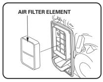
(b) After wetting the element by clean engine oil squeeze it tight by hand.
