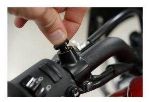
3. It may be necessary to lightly seat the plug with a RUBBER mallet. Apply any masking tape to the top of the plug to protect the finish and tap into place.
