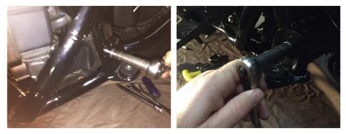
With the muffler off and out of the way you can remove the OEM muffler mounting bracket.
