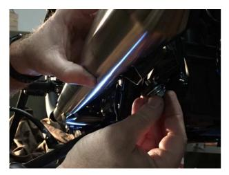
Now loosely install the bolt that secures the muffler to the frame mounting bracket.
