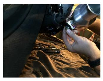
Once the muffler is seated, install the bracket mounts.
