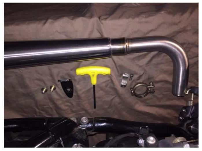
Here's a shot of the parts waiting to be installed. Included in the new muffler kit is a replacement bracket that will mount in the same location. You'll notice the picture shows the clamp that goes from the catalytic converter to the muffler. Hopefully you left it attached to the cat as described in upcoming scenes.
