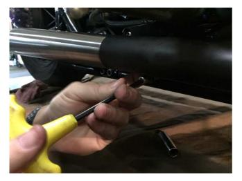
Attach the heat shield to the muffler. YOU"RE ENTERING THE HOME STRETCH!
