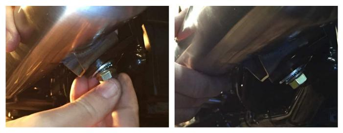
Here's are some closeups of the bolt, bracket, and muffler mounting bracket.
