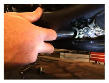
And again, just like on the left side, leave the catalytic converter clamp in place and gently work the muffler inlet into the gasket. However, on the right side now you will see why we loosened the header. You almost need three hands at this point. You need to guide the muffler into the cat and clamp the muffler to the heat shield in the same motion in order to get things properly aligned. Be patient, you can do it!
