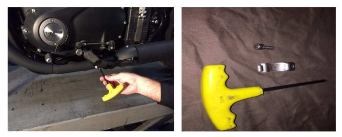
Remove the left side heat shield by loosening the clamp. It is located roughly under the left footpeg.
