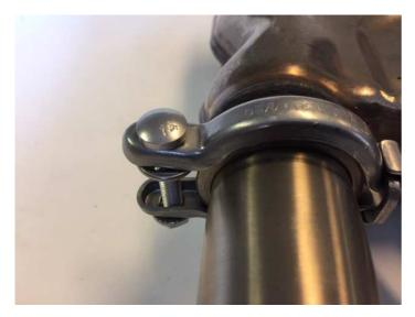
The depth that you will insert it into the gasket can vary. The alignment of the muffler to the mounting bracket is really what determines the depth, Tighten the clamp just a little since you may need to still do some aligning of the mufflers.
