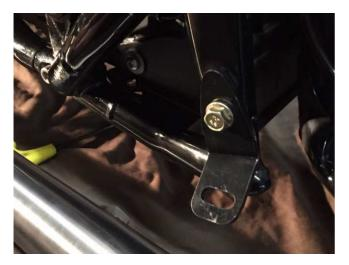
Bracket is installed on frame.
