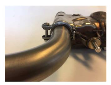
Now, gently work the edge of the muffler inlet into the graphite gasket. The muffler inlet has a beveled edge to help engage the muffler inlet into the gasket without causing damage. Rotate the muffler and gently wiggle it to get it in there.
