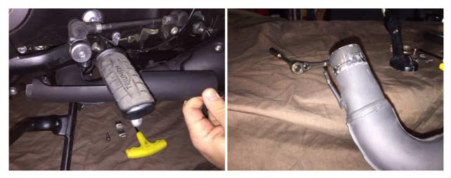
After removing the heat shield you should now be able to remove the muffler by gently wiggling it out of the catalytic converter clamp. If it won't come off, VERY CAREFULLY loosen the clamp just a bit more. You want to avoid taking the clamp completely off. Also, do not damage to the internal graphite gasket that the clamp is holding in place.
