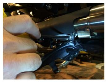
Install the heat shield clamp and bolt over the muffler inlet tube. Only tighten loosely for now.
