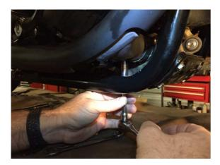
After you have loosened the header at the cylinder head, now loosen it on the right side clamp to the header crossover tube.
