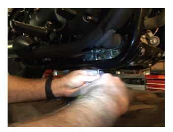
Now as on the left side, slightly loosen the clamp on the catalytic converter.
