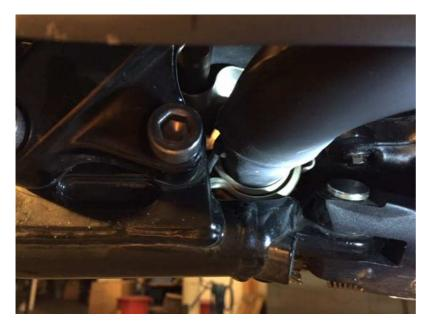
First, locate the clamp holding the muffler inlet to the catalytic convertor. DO NOT REMOVE CLAMP! It is very difficult to reinstall once completely removed. What you're going to do is loosen it just enough to be able to slide the muffler out. So at this point you're going to just loosen the nut a couple of turns.
