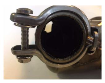
Now get ready to install the inlet of the muffler into the catalytic converter. Remember when we removed the OEM muffler we didn't remove the clamp, we just loosened it. Now is when you're going be grateful that you followed the directions. If you didn't follow the directions you will need to reinstall the gasket, flanged sleeve, and clamp BEFORE trying to mount the muffler inlet.
