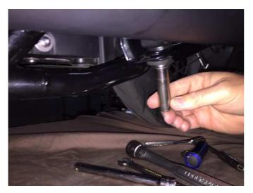
Now remove the bottom bolt that holds the muffler to the frame mounting bracket.
