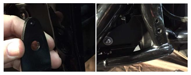
Make sure to align the nub on the new bracket lines up into the with the top hole on the frame.
