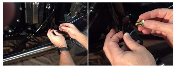
The upper hole secures the bracket to the frame using the supplied bolt and a star washer. Just loosely tighten all fasteners until the full system is installed and aligned.
