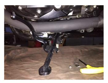
Lowering the kickstand makes it easier to remove the heat shield.
