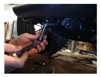
And remove the bolt holding the muffler to the frame bracket. You should now be able to lift the muffler away from the bike. Take notice of how the muffler clamps to the heat shield. You're starting to see why we loosened up the header at the cylinder head.
