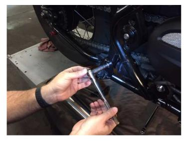
After you have removed the muffler you can now remove the rear mounting bracket just as we did on the other side.
