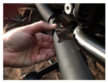
Begin the reinstallation of the heat shield, aligning it under the lip of the front/header heat shield.
