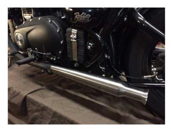
Don't tighten everything yet. You're now going to want to install the right side muffler and make sure the mufflers are level with each other before tightening everything down.
