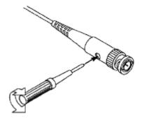
Figure 3-7 Adjust Probe
