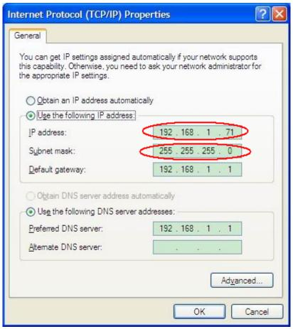
Figure 6-2 Set the network parameters of the computer
