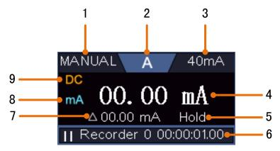
Figure 5-3 Multimeter Information Window
