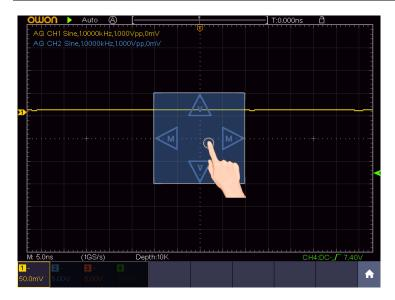
When the M and V icons appear, in the full screen, swipe left/right to change the time base, swipe up/down to change the voltage division of the selected channel. Click the icons to fine-turn, long-press to adjust continuously.
