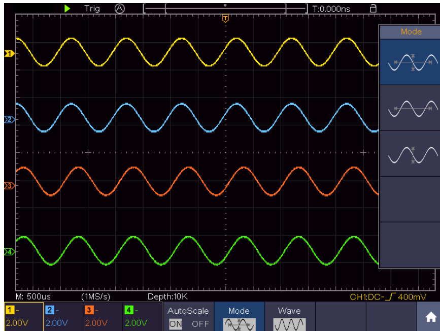
Figure 4-28 Autoscale Horizontal-Vertical multi-period waveforms
