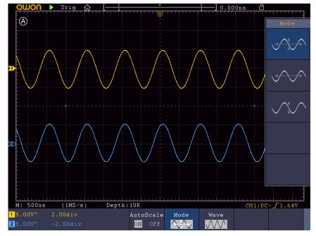
Figure 4-24 Autoscale Horizontal-Vertical multi-period waveforms
