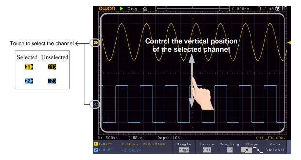
• Set the trigger level of the source in trigger menu (Trigger Level knob): Swipe up or down on the area nearby the trigger pointer on the right.
