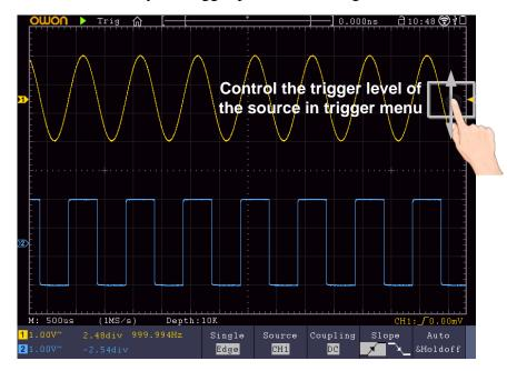
• Set the horizontal position (Horizontal Position knob): Swipe left or right on the display area.
