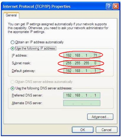
Figure 7-5 Set the network parameters of the computer
