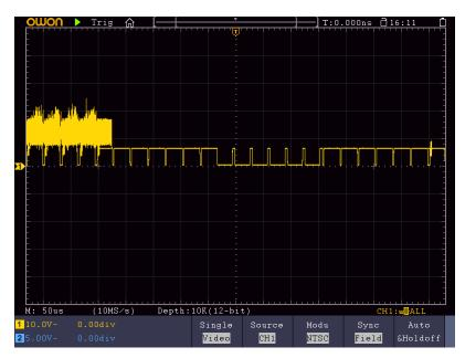
Figure 9-7 Waveform Captured from Video Field Trigger
