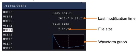
If a USB device is connected, and you want to save the waveform to it, select **Memory** in the right menu as **USB**. The instrument lists a directory of the folders and files on the USB memory device. Select a folder or file using the **M** knob to scroll up
