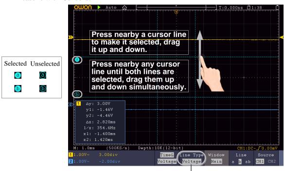
Switch horizontal or vertical lines If vertical lines are selected, drag left and right.
