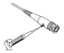
Figure 3-8 Adjust Probe
