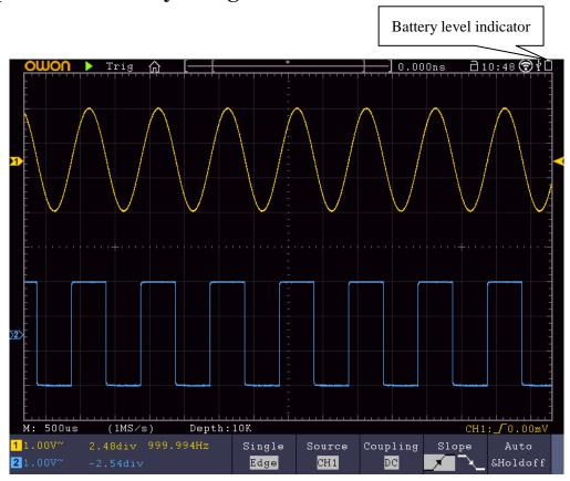
Figure 12-1 Battery level indicator
