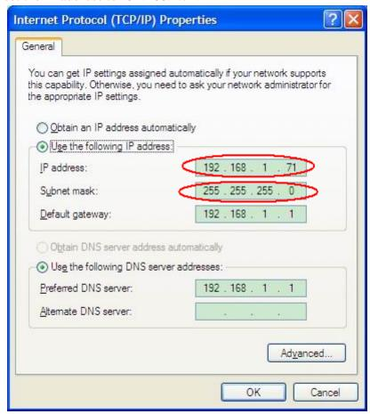
Figure 7-2 Set the network parameters of the computer
