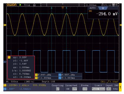
Figure 4-23 Time&Voltage Cursor Measurement
