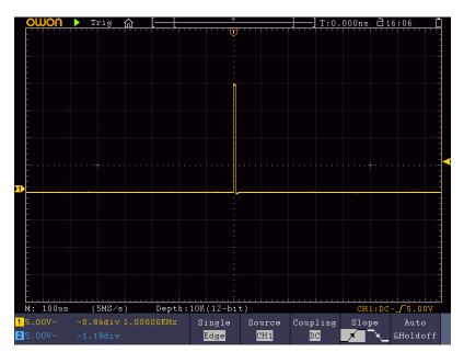
Figure 9-3 Capturing a Single Signal
