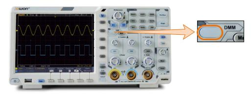
Figure 6-2 Multimeter Button
