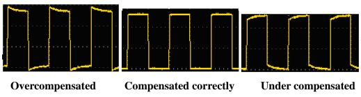
Figure 3-7 Displayed Waveforms of the Probe Compensation
