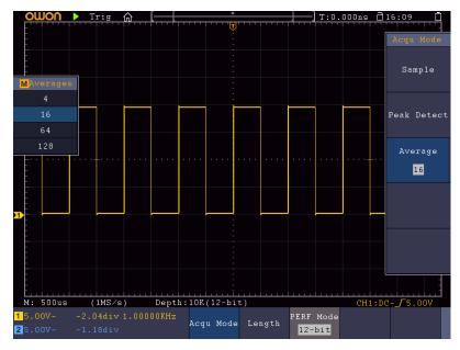
Figure 9-5 Reduce Noise level by using Average function
