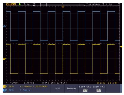
Figure 9-2 Waveform of Gain Measurement
