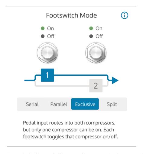
Press the left or right footswitches to toggle Comp 1 or Comp 2 on/off. Only one Comp can be on at a time.
