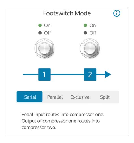
Press the left or right footswitches to toggle Comp 1 and Comp 2 on/off. One or both can be on at the same time. The output of Comp1 feeds the input of Comp 2
