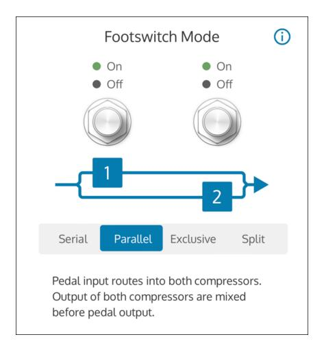
Press the left or right footswitches to toggle Comp 1 and Comp 2 on/off. One or both compressors can be on at the same time. The input signal is split before feeding into each Comp separately, and the outputs of both Comps are mixed before the pedal output.
