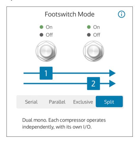
Press the left or right footswitches to toggle Comp 1 and Comp 2 on/off. One or both compressors can be on at the same time. Input 1 routes to Comp 1, and out of Output 1. Input 2 routes to Comp 2, and out of Output 2.
