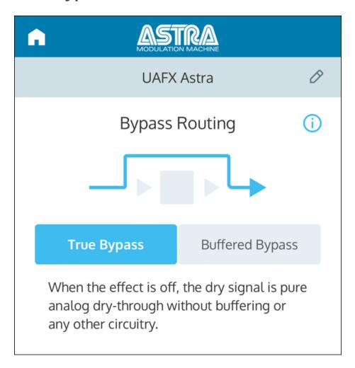
When bypass routing is set for true bypass and the effect is off, the dry signal is pure analog dry-through from input to output, without buffering or any other circuitry, via mechanical relays. By default, your UAFX pedal is set for true bypass.
