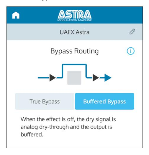
When bypass routing is set for buffered bypass, the output is buffered when the effect is on, and also when the effect is off.
