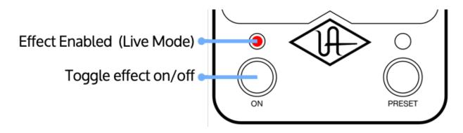
**In Live mode**, the sound reflects the current positions of the knobs, switches, and LEDs on the pedal, and the left footswitch toggles the Live mode effect on/off.
