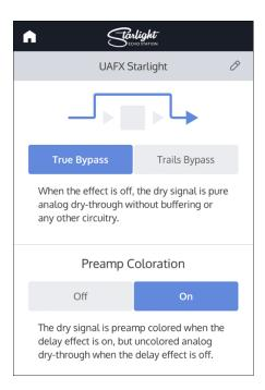
When preamp coloration is off, the dry signal is always uncolored and analog dry-through when the delay effect is on, and also when the delay effect is off, with both true bypass and trails bypass routings.
