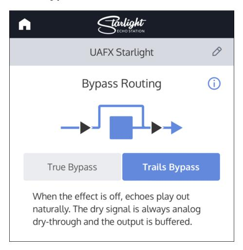
When bypass routing is set for trails bypass and the effect is off, delays play out naturally, rather than stopping suddenly.
