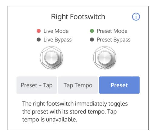
When set to preset, the right footswitch immediately loads the preset with its stored tempo, and toggles the preset on/off. Tap tempo is unavailable with this setting.
