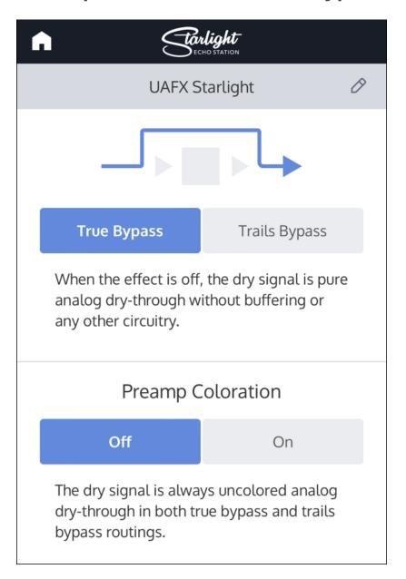
When preamp coloration is on and bypass routing is set for true bypass, the dry signal is preamp colored when the delay effect is on, but uncolored analog dry-through when the delay effect is off.
