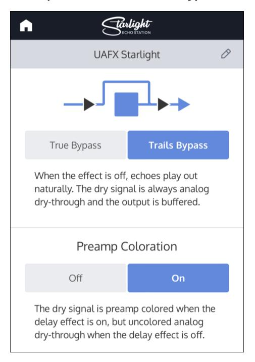
When preamp coloration is on and bypass routing is set for trails bypass, the dry signal is preamp colored when the delay effect is on, and also when the delay effect is off.
