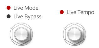
When set to tap tempo, the right footswitch taps quarter note tempo for Live mode only. The right footswitch LED blinks red at the current tempo. Although you cannot access the stored preset in this mode, its settings remain intact.
