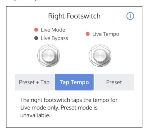
When set to tap tempo, the right footswitch taps quarter note tempo for Live mode only. The right footswitch LED blinks red at the current tempo. Although you cannot access the stored preset in this mode, its settings remain intact.
