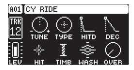
**TUNE** (Tune) sets the pitch of the interacting oscillators that make up the ride cymbal model. **TYPE** (Cymbal Type) selects different sets of fundamental oscillator frequencies, as well as different inter-oscillator logical interaction. (A-D)
