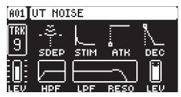
**SDEP** (Sweep Depth) sets the depth of the LP Filter sweep. Negative as well as positive sweeps are possible.
