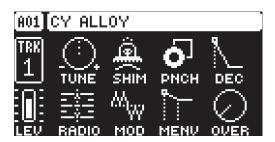
**TUNE** (Tune) offsets the incoming note value. This parameter is bipolar. A setting of 0 leaves the pitch unchanged.
