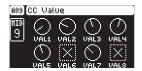
VAL1-VAL8 (CC 1–8 Value) controls the values that the CC commands send. You specify the CC commands themselves on the AMP (CC SELECT) page. These parameters default value is OFF. Press [FUNC] + DATA ENTRY knobs to activate the parameters and then turn the DATA ENTRY knobs to set a value. (OFF, 0–127)
