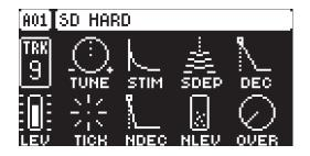
TUNE (Tune) sets the pitch of the oscillators. The interval between them is fixed.
