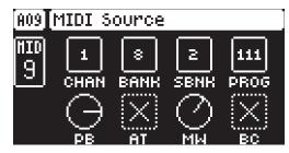
**CHAN** (Channel) sets the MIDI channel the track sends MIDI data to. If you set this parameter to OFF, it turns the MIDI track off. Please note that this parameter cannot be parameter locked. (OFF, 1–16)
