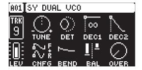
TUNE (Osc 1 Tune) sets the tuning of oscillator 1.
