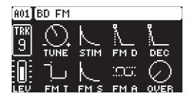
TUNE (Tune) sets the pitch of the first (modulated) oscillator.
