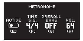
ACTIVE activates/deactivates the metronome. You can also press [FUNC] + [PTN] to toggle the metronome on and off when you are not in the METRONOME menu. TIME SIG. controls the note and beat measure of the metronome time signature.
