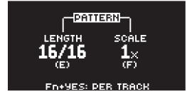
**LENGTH** controls the step length of the pattern. The leftmost number displays the number of steps in the pattern. The total length, displayed by the second number, determines the maximum number of steps available in the pattern. If you use 17 steps or more in a pattern, the **[PAGE]** key is (while in GRID RECORDING mode) used to toggle between the different pattern pages.
