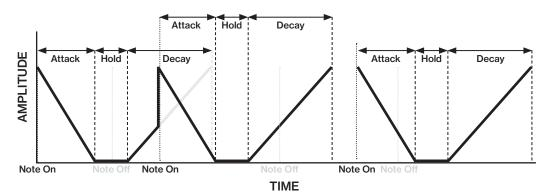
Inverted amplitude envelope with HOLD set to NOTE.
