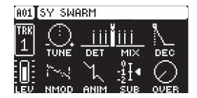
**TUNE** (Tune) offsets the incoming note value. This parameter is bipolar. A setting of 0 leaves the pitch unchanged.
