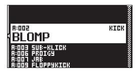
The SOUND BROWSER is used to preview and load sounds. You can also press [FUNC] + *LEVEL/DATA* to open the SOUND BROWSER. This menu will show a list of all sounds in the +Drive sound library that can be loaded to the active track. Scroll the list by turning the *LEVEL/DATA* knob or by pressing [UP]/ [DOWN]. Press [TRIG 9–16] to select sound bank A–H. Press [FUNC] + [YES] to preview the sound before you load it to the track. You can also use KEYBOARD mode, or an external MIDI controller, sending
