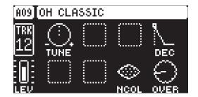
TUNE (Tune) sets the pitch of the oscillators of the open hihat.
