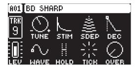
TUNE (Tune) sets the pitch of the oscillator.
