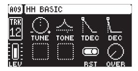
TUNE (Tune) sets the pitch of the six oscillators that combine to make the basic hihat sound.
