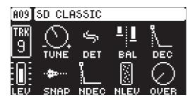
**TUNE** (Tune) sets the common pitch of the oscillators.
