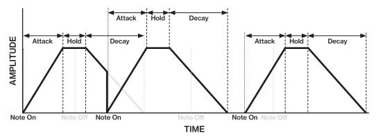
Amplitude envelope with MODE set to AHD and HOLD set to NOTE.
