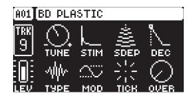
TUNE (Tune) sets the pitch of the two interacting oscillators.
