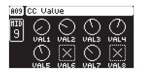
VAL1-VAL8 (CC 1–8 Value) controls the values that the CC commands send. You specify the CC commands themselves on the AMP (CC SELECT) page. These parameters default value is OFF. Press [FUNC] + DATA ENTRY knobs to activate the parameters and then turn the DATA ENTRY knobs to set a value. (OFF, 0–127)
