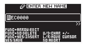
The [LEFT] and [RIGHT] arrow keys are used to navigate between the characters. Turning the *LEVEL/ DATA* knob or pressing the [UP] or [DOWN] arrow keys selects the characters. [FUNC] + [NO] erases characters. [FUNC] + [YES] inserts space. Press and hold [FUNC] to access the Pop-up Naming menu.
