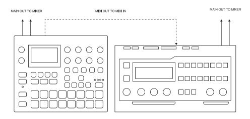
Syntakt has extensive capabilities to use its sequencer's MIDI tracks to control other MIDI-equipped synthesizers.
