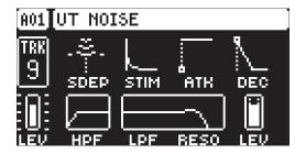
**SDEP** (Sweep Depth) sets the depth of the LP Filter sweep. Negative as well as positive sweeps are possible.
