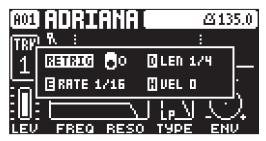
RETRIG Turns the retrig lock ON/OFF. Use DATA ENTRY knob A to turn retrig on/off.
