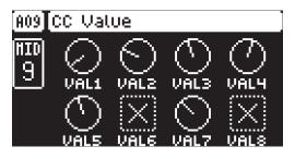
VAL1-VAL8 (CC 1–8 Value) controls the values that the CC commands send. You specify the CC commands themselves on the AMP (CC SELECT) page. These parameters default value is OFF. Press [FUNC] + DATA ENTRY knobs to activate the parameters and then turn the DATA ENTRY knobs to set a value. (OFF, 0–127)
