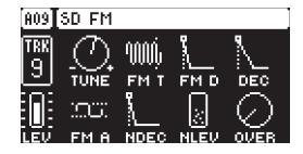
TUNE (Tune) sets the pitch of the first (modulated) oscillator.
