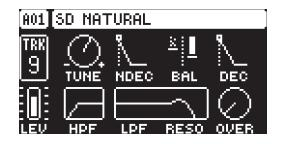
TUNE (Tune) sets the pitch of the first oscillator.
