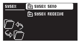
When receiving or sending SysEx data, the MIDI ports or the USB port of the Syntakt should be connected to the external sending/receiving device.
