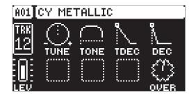
**TUNE** (Tune) sets the pitch of the ring-modulated oscillators of the metallic cymbal. **TONE** (Tone) sets the tone of the metallic transient.
