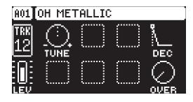
TUNE (Tune) sets the pitch of the interacting oscillators of the metallic hihat.
