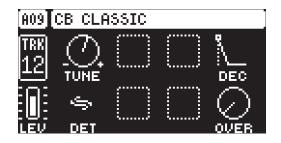
TUNE (Tune) sets the base pitch of the two oscillators.
