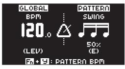
Turn DATA ENTRY knob E to set the SWING ratio to 51-80%. The default setting is equal spacing, 50%.
