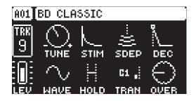
TUNE (Tune) sets the pitch of the oscillator.
