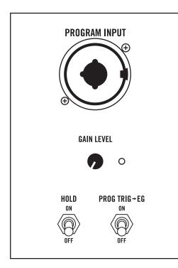
The **PROGRAM** section of Spectravox sends the signal connected to the **PROGRAM INPUT** into the analysis filter bank—whose outputs are the 10 envelope followers (**1 ENV F, 2 ENV F ... 10 ENV F**). The **PROGRAM** signal thus animates the synthesis filter bank when Spectravox is in **VOCODER** mode.
