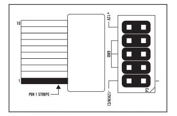
5. Look at the back of your Spectravox. There is a 10-pin power header on the back of the PCB that accepts a 10-pin Eurorack power ribbon cable (not included).
