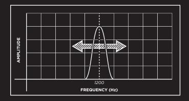
Spectravox is a unique exploration of the topology of the vocoder due to its filter design. Whereas most previous analog filter banks have their filters fixed in place, all 10 filters of Spectravox can be shifted up and down the frequency spectrum! Additionally, its filters all have variable **RESONANCE**, which provides for colorful sound design possibilities.
