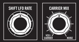
Move **SHIFT LFO RATE** up to increase the **LFO** rate, and move it down to decrease. Set the **SHIFT LFO RATE** down around eight o'clock and increase the **SHIFT LFO AMT** to around two o'clock to hear wide comb filter animation akin to a phaser effect. Shift the **CARRIER MIX** knob all the way counterclockwise to **VCO/CARRIER** to hear just the VCO, and as you move **RESONANCE** up you will hear a kaleidoscopic resonant sweep.
