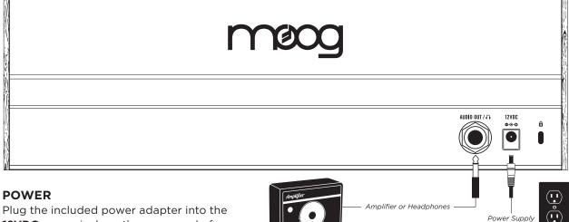
12VDC power jack on the rear panel of your Spectravox.
