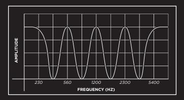
Play again with **RESONANCE** and **SPECTRAL SHIFT**. You will notice that all five filters move as you turn **SPECTRAL SHIFT**! This is the unique power of Spectravox: its filters are not fixed, but moveable.
