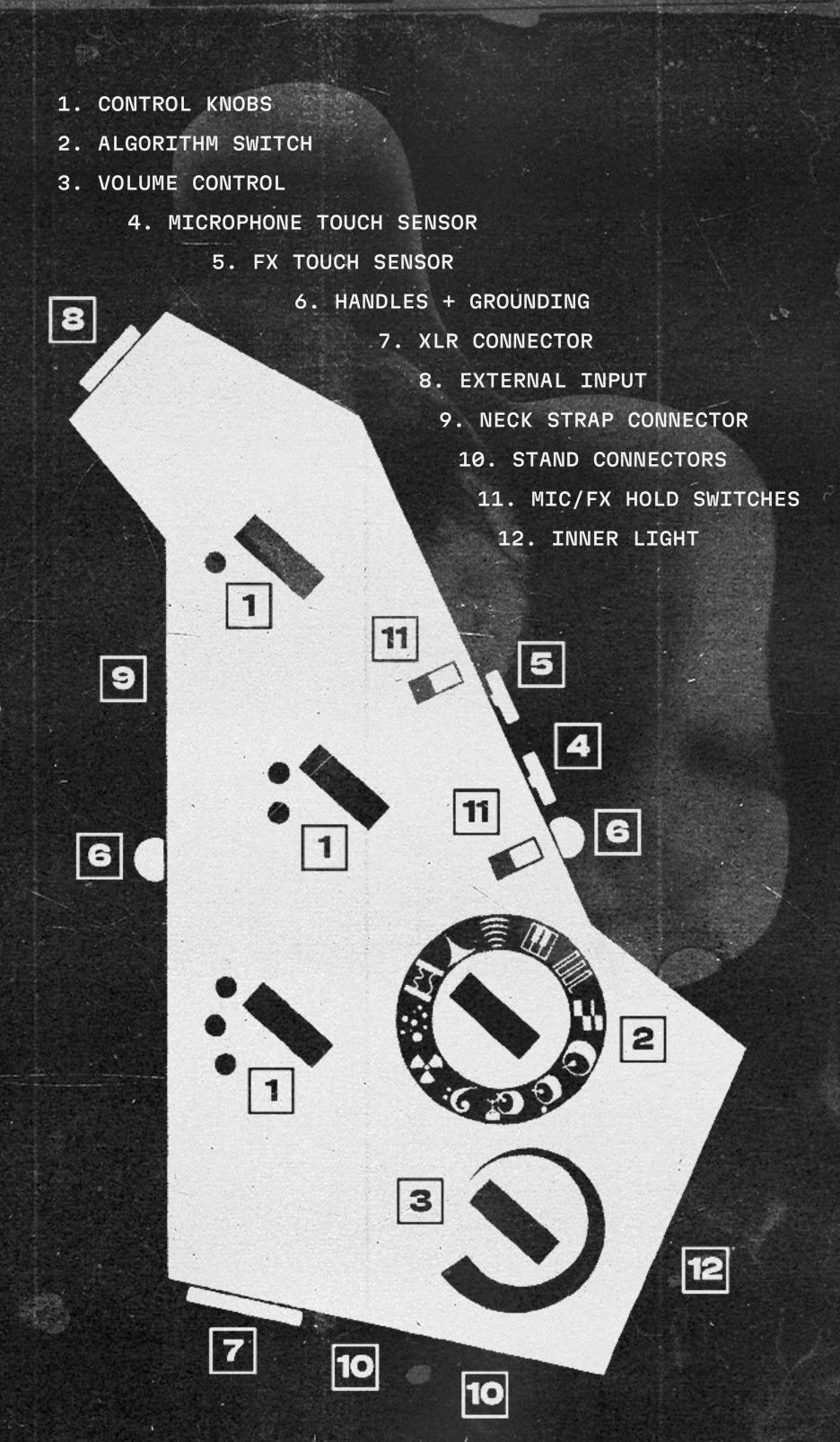
1 Control knobs for synthesis and processing parameters
