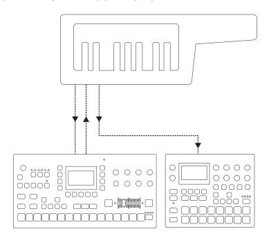
The MIDI OUT of an external synthesizer is connected to the Octatrack MKII MIDI IN. The Octatrack MKII MIDI OUT is connected to the MIDI IN of the synthesizer. A synth module is connected to the MIDI THRU of the synthesizer. The Octatrack MKII can MIDI control both the synthesizer and the synth module. At the same time the keyboard of the synthesizer can be used to play Octatrack MKII samples, play the synthesizer itself as well as the synth module.
