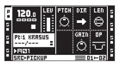
**PITCH** adjusts the pitch of the sample. The max setting pitches the sample up an octave, a min setting pitches the sample down an octave. Integer changes are equivalent to semitones. For overdubbing and replacing to be possible, this parameter must be set to 0.
