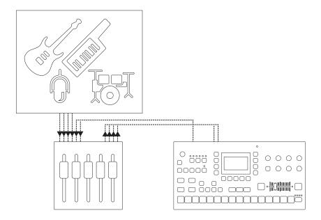
Four mixer aux sends are connected to the inputs of the Octatrack MKII. Each aux send sends a different signal. The Octatrack MKII applies effects, reconstructs the incoming audio and sends back the real-time processed audio to the stage mixer.
