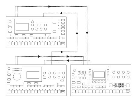
A Machinedrum and a Monomachine are MIDI slaved and connected to the two input pairs of the Octatrack MKII. The Octatrack MKII acts like a super mixer. It adjusts the levels of the incoming signals, applies effects and samples the other machines in real time. Two main methods setting up the Octatrack MKII exist. It can either listen to the incoming audio by using the DIR parameters of the MIXER menu or by using Thru machines.
