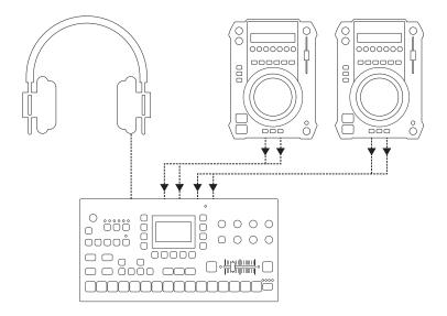
Two DJ decks are connected to the Octatrack MKII inputs. The headphones output is set to monitor both the main and cue outputs. The crossfader is assigned to control the main output balance between the two incoming signals. The Octatrack MKII can mix between the DJ decks by either using the DIR method or the Thru machines method.
