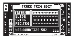
Pressing [YES] while in this menu can be used to quantize trigs to approximately 50 percent of their original micro timing value. Use this operation when you want to tighten up a track where micro timing has been used, but not fully quantize it. Quickly perform the operation 6 times in a row to have the micro timing cleared for all trigs. Read more about micro timing in the section "12.12 MICRO TIMING" on page 76
