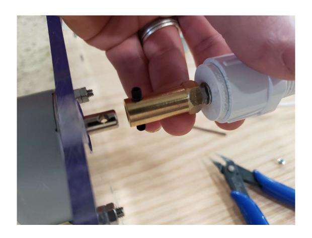
Use the larger allen wrench to remove the 2 screws holding the motor to the plexiglass.
