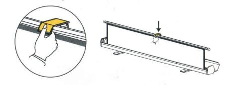
Close the casing and then rotate the left and right support plate to 90 degree.
