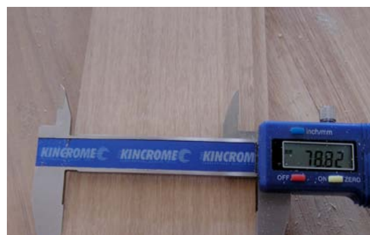
Corrected moisture meter reading is 15% and the board cover width is 78.82 mm. The higher reading and narrow cover width can indicate even higher moisture content when manufactured.
