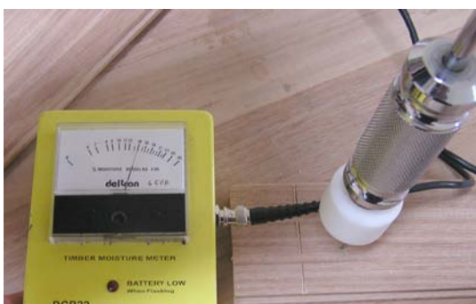
Corrected moisture meter reading is 15% and the board cover width is 78.82 mm. The higher reading and narrow cover width can indicate even higher moisture content when manufactured.
