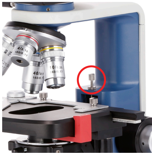
[image: adjusting height limit]
