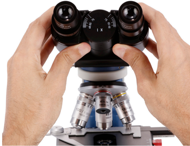
[image: adjusting ocular tubes]
