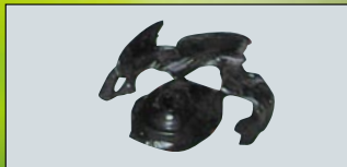
Impeller made of ordinary ABS resin After 24 hours of pump operation Loss of impeller weight:46%
