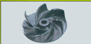
Impeller made of engineering plastic After 200 hours of pump operation Loss of impeller weight:3.3%
