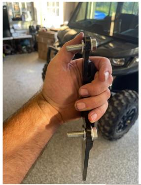
Ensure tire and wheel are removed. Once tire and wheel are off, remove these 2 bolts.
