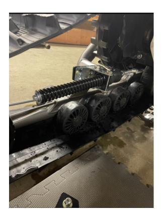
Start with 1 rear bracket (interchangeable and not side specific).
