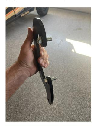
Remove caliper bolts. Line bracket into place on spindle, and tighten down the flange bolts using a wrench to secure the caliper/bracket.
