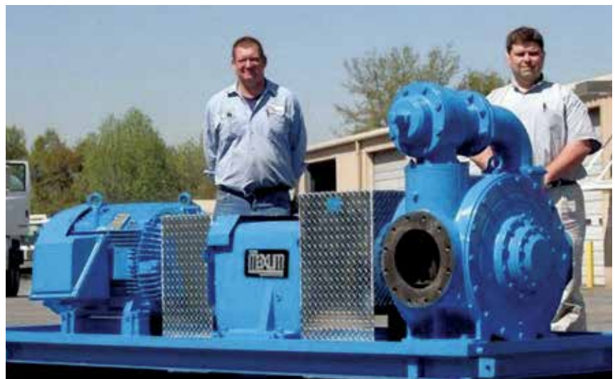
Blackmer Pump, HXL-12, 100 HP, 2200 GPM
