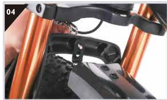
Note that the headlight and the fender share a screw
