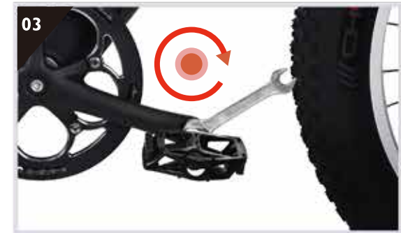
03 The installation direction of the R pedal is clockwise, and tighten it toward the front wheel.
