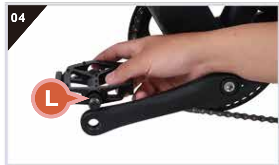
04 “ L” pedal installation is on the left side. As shown.
