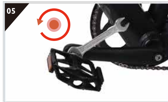
05 The installation direction of the L pedal is counterclockwise, and tighten it towards the front wheel
