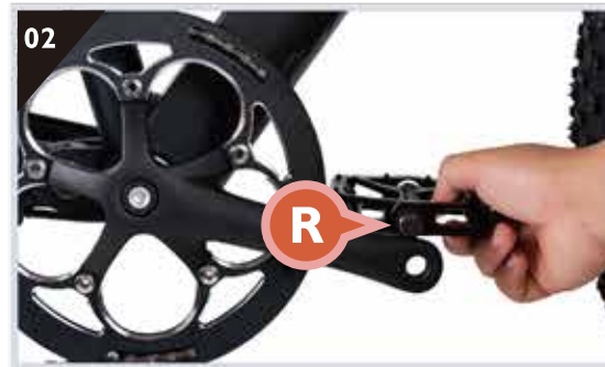
02 “ R” pedal is installed on the right (crankset) side. As shown.
