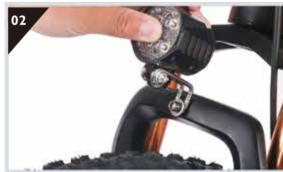
Pass the screw through the front light and fix it to the fork
